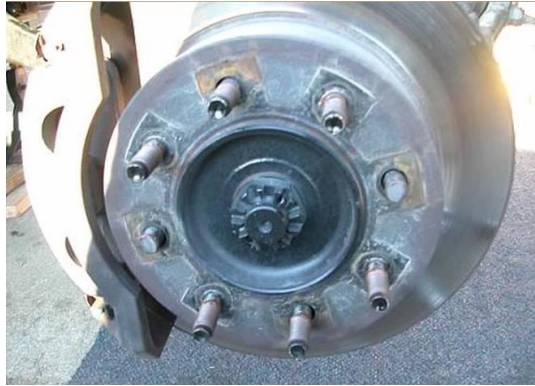
Results of Over Tightening the wheel nuts
