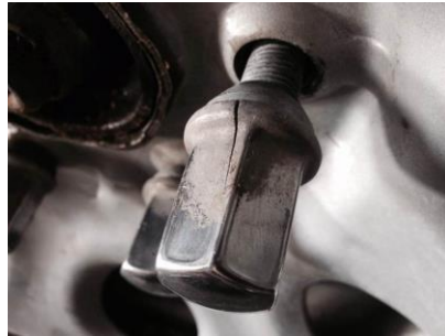
Wheel nut cracked
