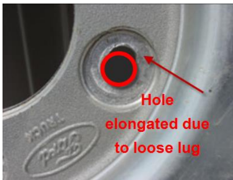
Wear due to lug nut being loose while in motion
