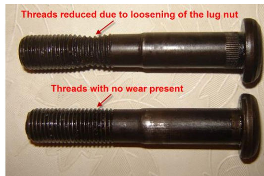
Wear due to lug nut being loose while in motion
