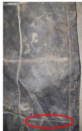
• Punctured, severed or missing braid elements are not acceptable
