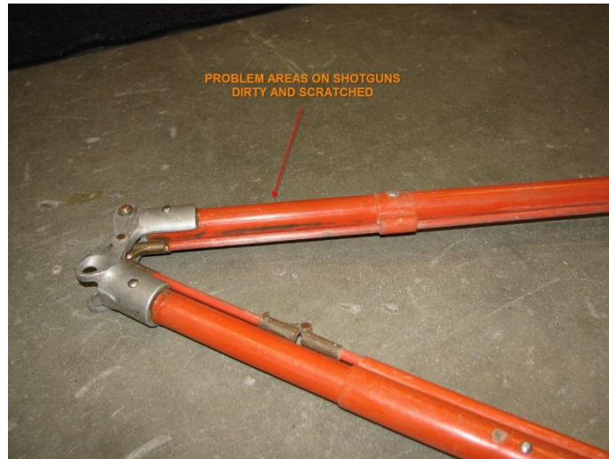
Figure#5 - Dirt and Contamination on Stick
