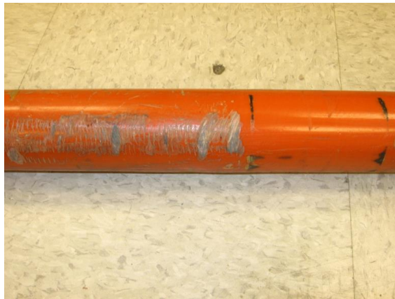
Figure#3 - Damaged Fiberglass (Deep Rub Marks)
