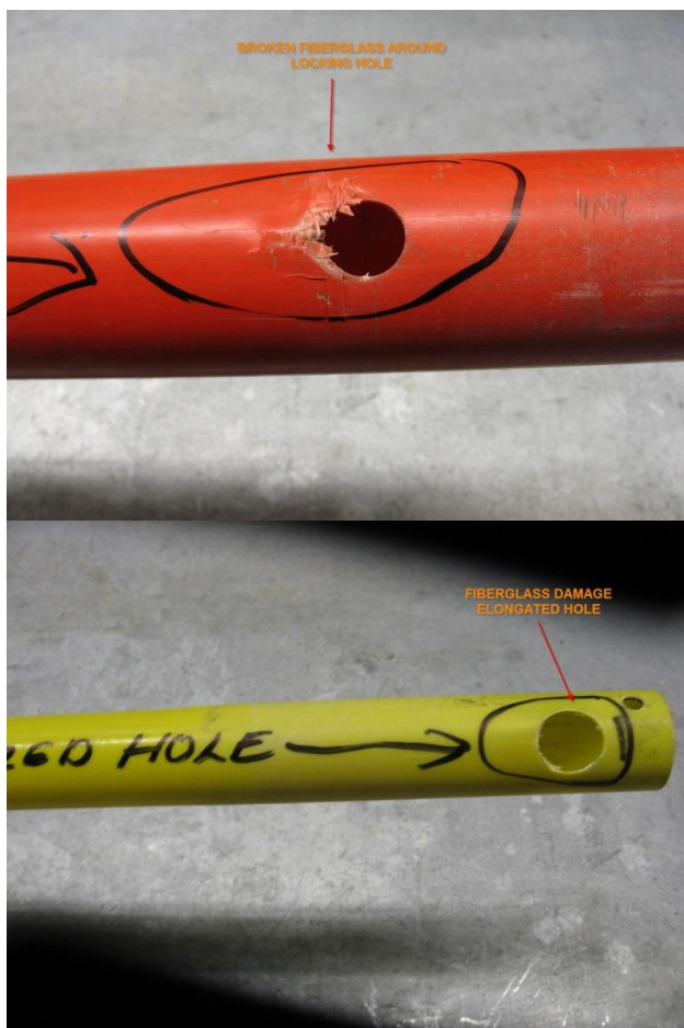
Figure#4 - Damaged Locking Hole
