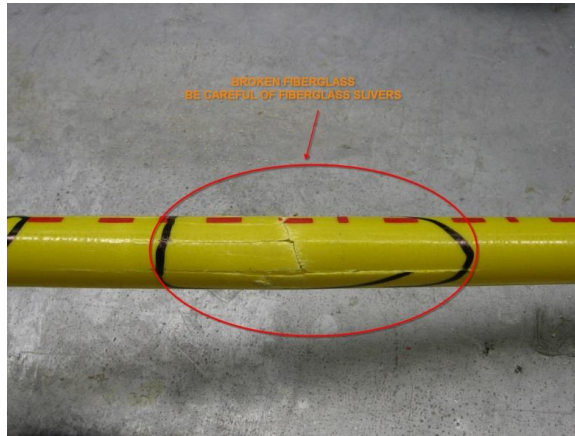
Figure#2 - Broken Fiberglass
