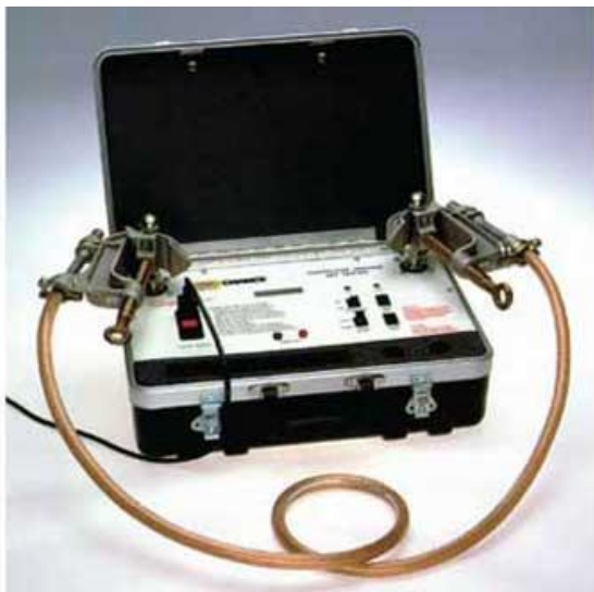
Figures #8 & #9 Test set up with bond and ground assemblies
