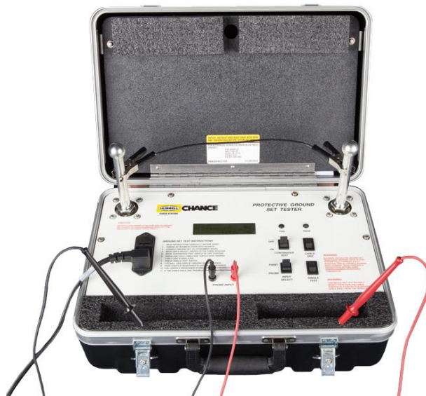
Figure #7 Chance Protective Ground Set Tester Self Test Setup
