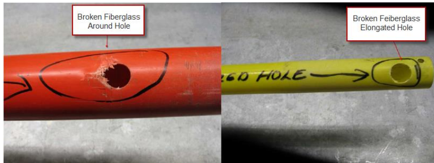
Figure #4 Damaged Button Hole
