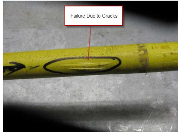
Figure#1 - Cracks in the Fiberglass
