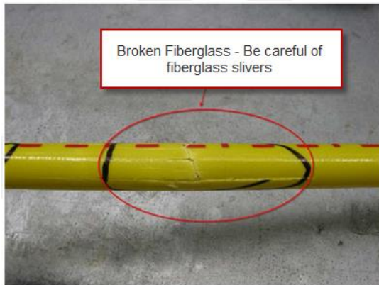
Figure#2 - Broken Fiberglass
