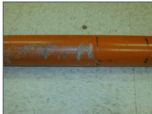
Figure#3 - Damaged Fiberglass (Deep Rub Marks)
